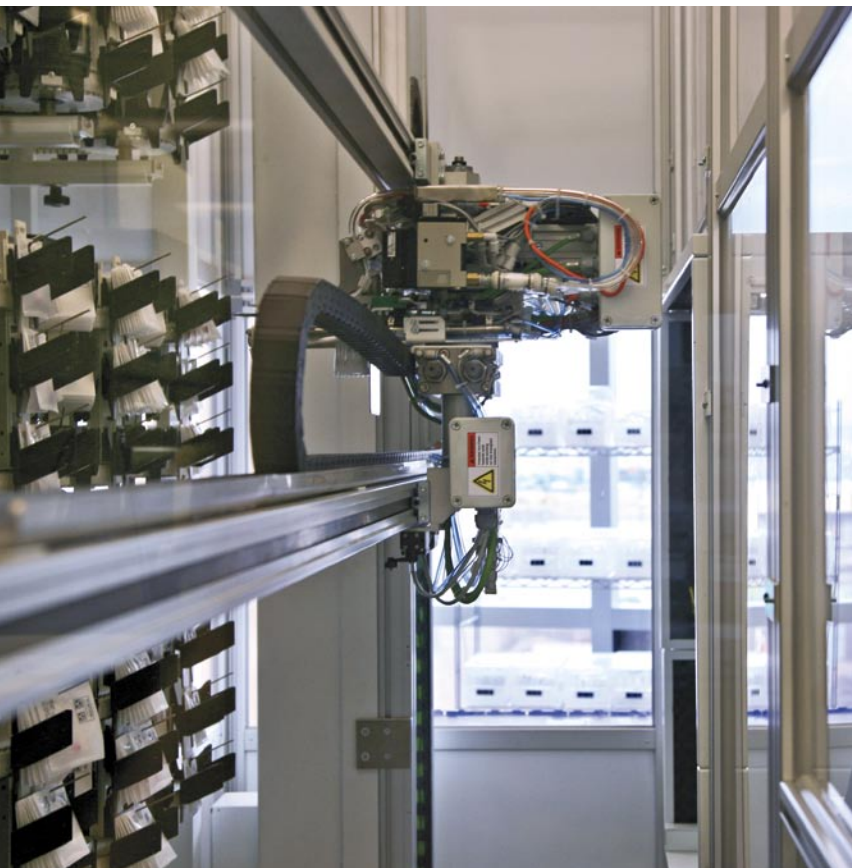
A robotic “pill picker” selects, packages and dispenses individual doses of pills.
